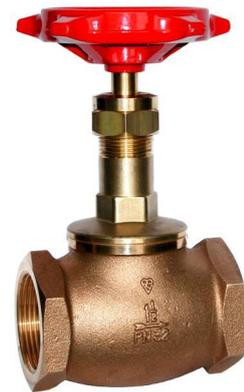
This robustly manufactured screwed bonnet globe valve with a PTFE valve disc is ideally suited for isolation duty, providing a leak-tight shut off with the capability of being used partially open to regulate flow.
