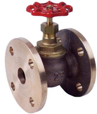
An economical globe valve with a PTFE valve disc which is ideally suited for isolation duty, providing a leak-tight shut off with the capability of being used partially open to regulate flow.
