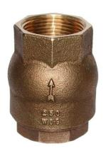
A superior spring-loaded non-return valve with a bronze body and P.T.F.E. seals which makes this valve particularly suitable for low-pressure steam applications and marine environments. This valve requires a minimum pressure of 0.04 bar to open and can be installed in both horizontal and vertical lines with upward flow or in any intermediate position.
