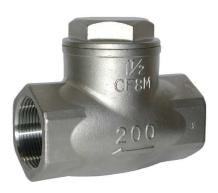
An economic stainless steel swing type check valves suitable for steam, water and oil applications. It can be fitted in the horizontal position or in the vertical position with the flow going upwards. This valve requires a low minimum pressure to open.
