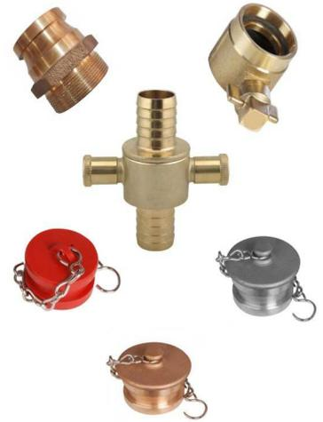
The BS 336 Instantaneous coupling system connects using a spring loaded catch mechanism on the female section of the coupling. They are widely used in water hydrants and firefighting applications in the United Kingdom.
